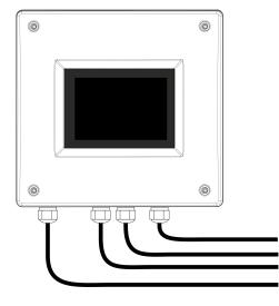
To prevent water from running into the DOL 100 via cables and screwed connections, run the cables so that water does not gather around the cable in the gasket of the screwed connection.
