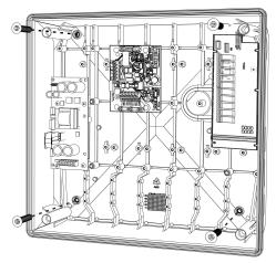
Mount the DOL 100 digital box on the wall using four screws.
