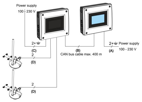
(A) Power supply to the controller two-wire cable including earthing contact.
